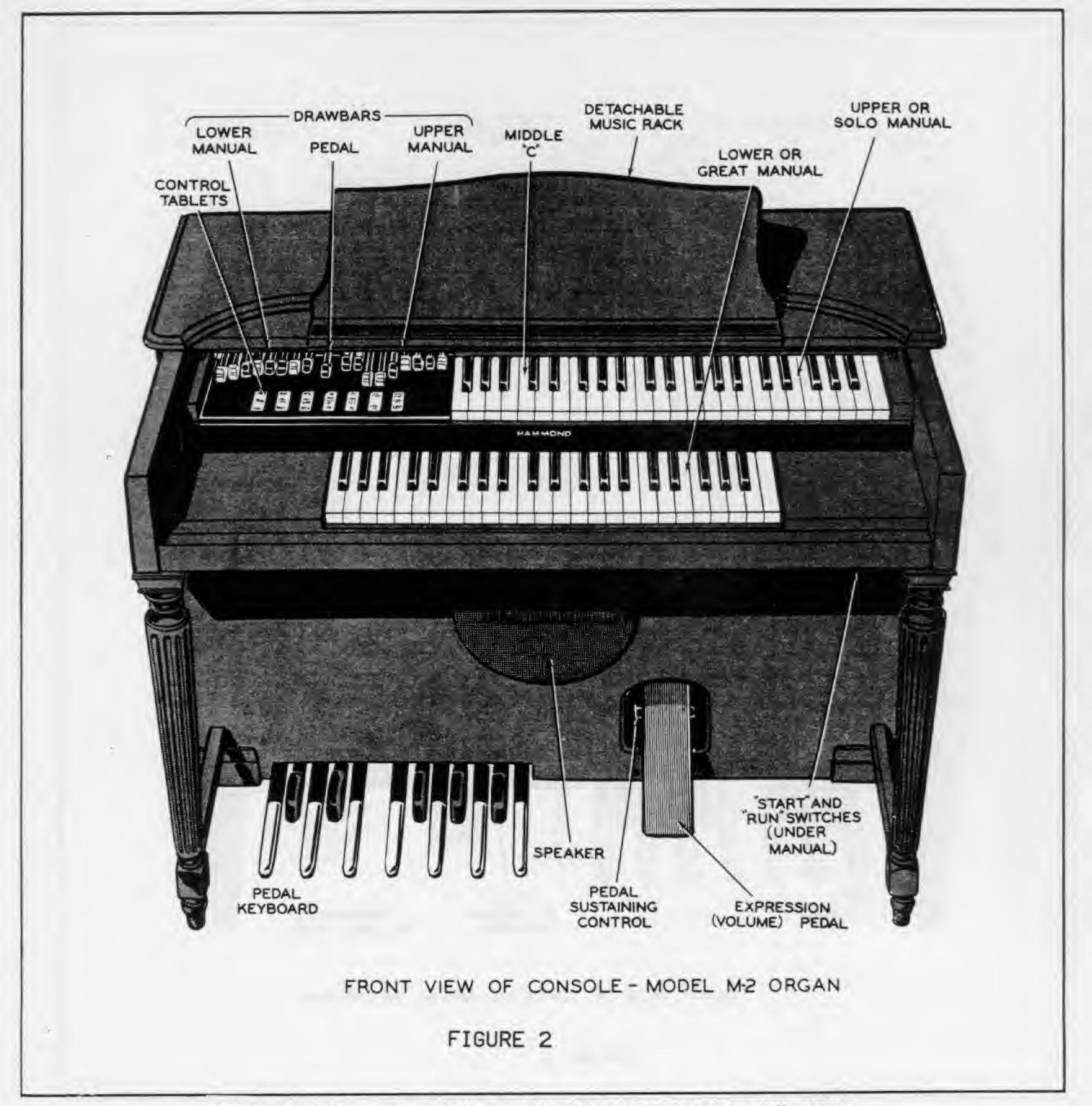
DIMENSIONS: 45-5/8" WIDE; 25-3/8" DEEP; 42" HIGH AC INPUT: 103 WATTS OUTPUT: 11 WATTS E.I.A. WEIGHT: 249 LBS.
